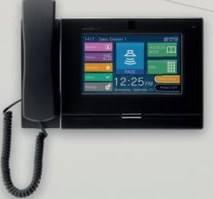
Combining video entry security, internal communication, emergency stations and multicast paging.
